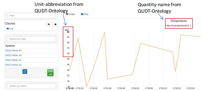
Figure 2 Temperature observation rendered in MOSCITO with help of the semantic information
