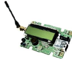
Figure 1. FOKUS Sensor Board
