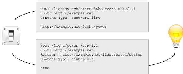
Figure 1. Example of how an observer is added to a resource (top) and how that resource notifies its observers when its value changes (bottom).
